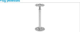
GIFAfloor Plug pedestals M16 ST and M20 ST are made of galvanised steel. The foot part consists of a tube with a wall thickness of 2.0 mm and a welded-on foot plate. The head section consists of an M16 or M20 threaded rod with a welded-on head plate. The height is adjusted by means of the screw nut resting on the tube. Minimum insertion depth of the threaded rod in the tube is 20 mm. After adjustment secure against height change with Knauf GIFAfloor pedestal lock EC 1.
