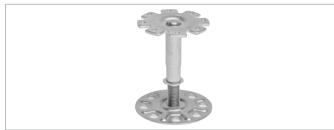
GIFAfloor Thread pedestals M16 S are made of galvanised steel. The foot part consists of an M16 threaded rod with foot plate. The head part consists of a tube with a wall thickness of 2.0 mm with internal thread and a welded head plate. The height of the thread pedestals is adjusted by turning the pedestal head. Minimum screw-in depth (=thread length of the tube) 15 mm. After adjustment secure against height change with Knauf GIFAfloor pedestal lock EC1.
