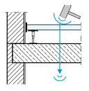
Standard flank impact sound level  $L_{n,f,w}$ The standard flank impact sound level  $L_{n,f,w}$  indicates the impact sound transmission via the raised floor construction from one room to the neighbouring room. The lower the weighted standard flank impact sound level  ${\rm L}_{\rm n.f.w}$  the better the horizontal impact sound insulation of the installed raised access floor.
